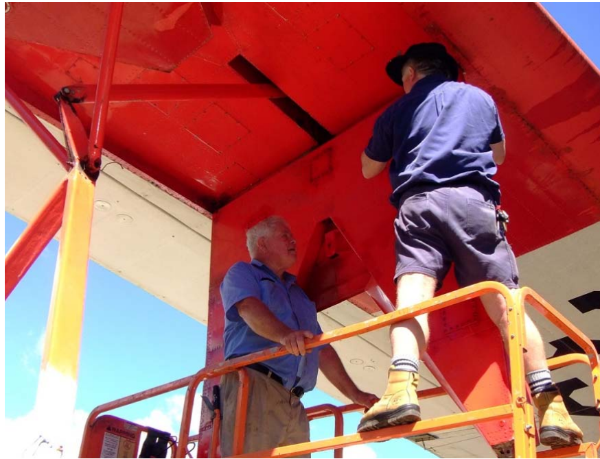
David Sieber (L) and Roger Matthysen (R) immediately following the attachment of the right-hand float pylon to the wing
