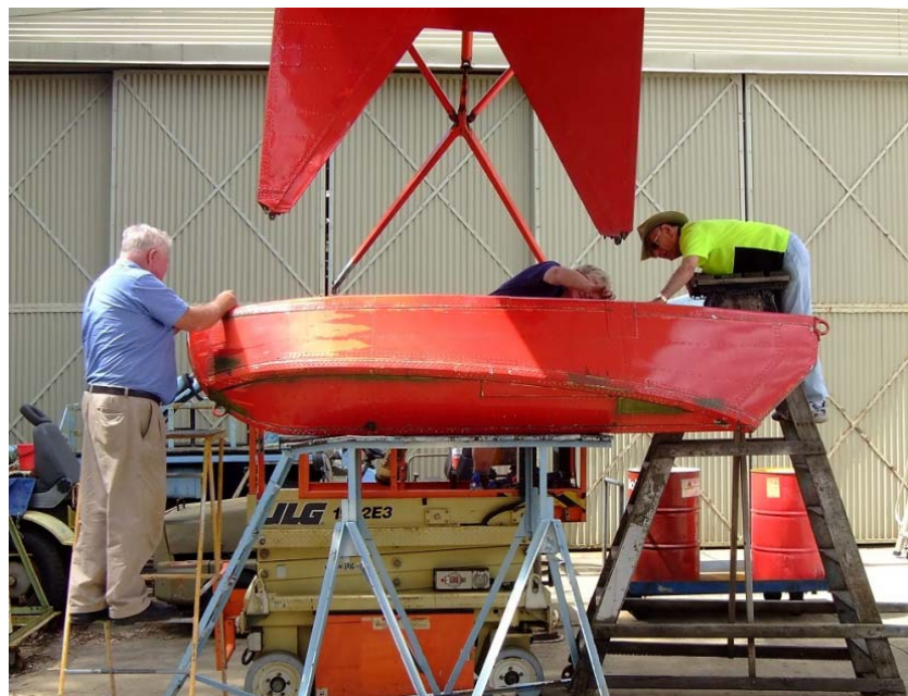
L-R: David Sieber, Roger Matthysen and Len Linfoot readying the right-hand float for attachment to the float pylon
