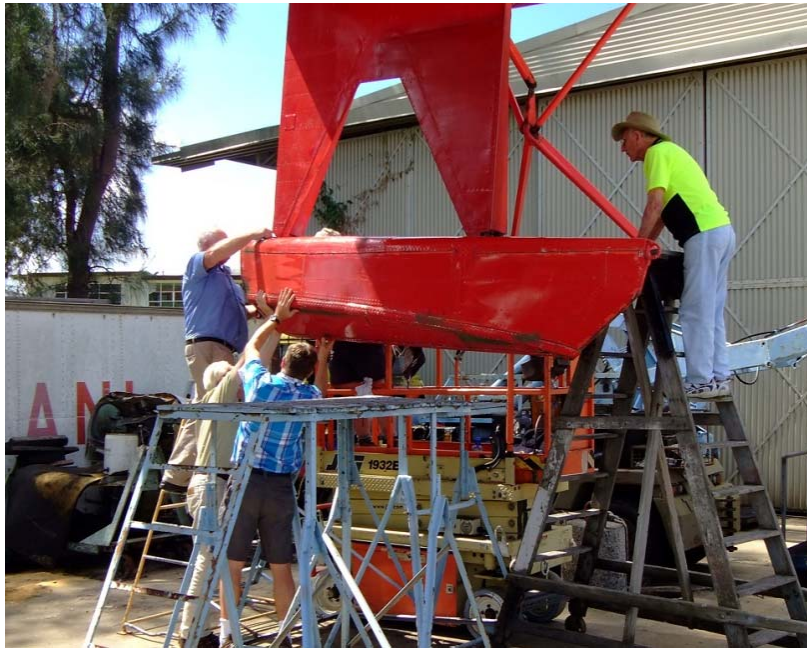
Contact! The right-hand float is re-attached to the float pylon. L-R: David Sieber, Spencer Ferrier, Malcolm Burns, Len Linfoot (Roger is hiding behind the float)
