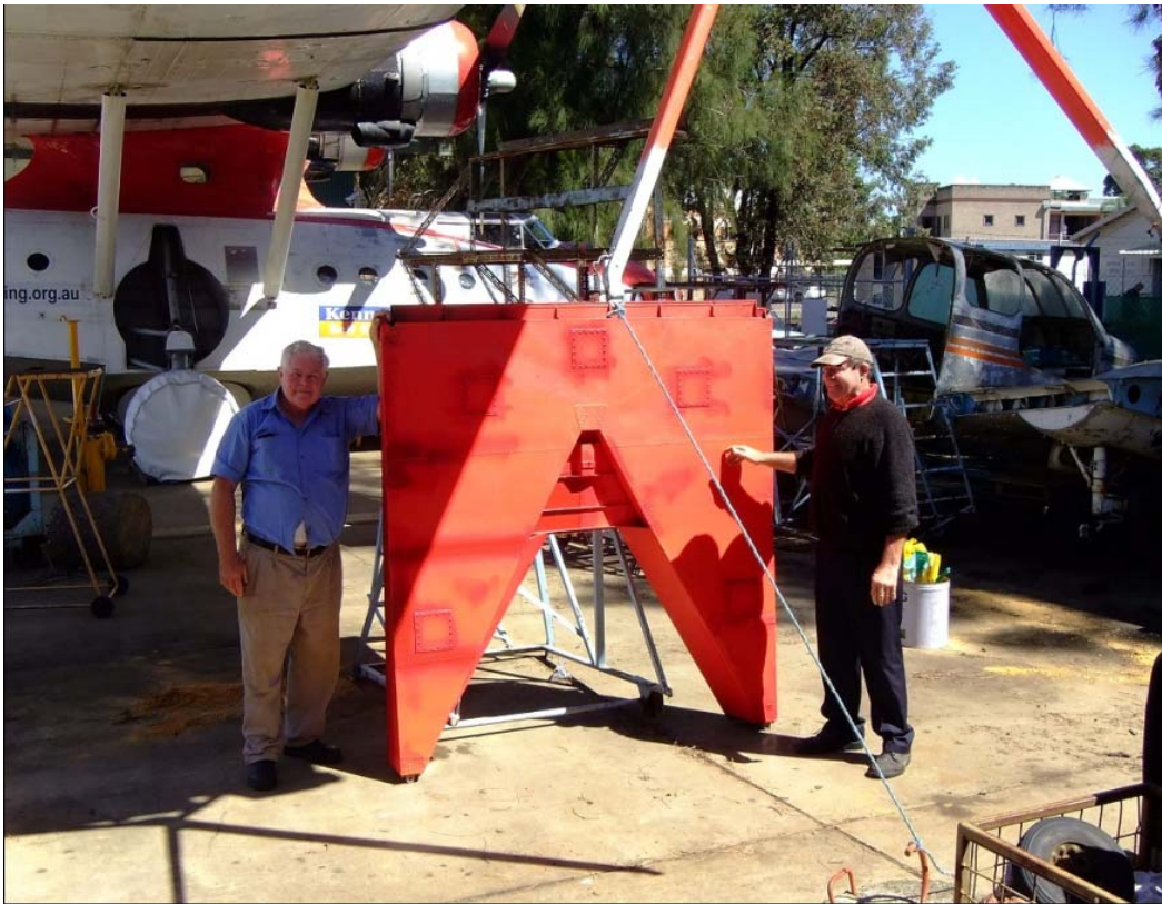
David Sieber (L) and Patrick O'Hara (R) proudly standing with the right-hand float pylon immediately prior to its attachment to the wing
